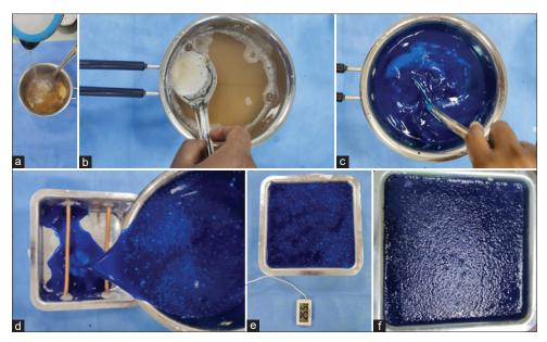
Figure 2: Preparation and settlement of the mixture. (a) Pouring lukewarm water into the gelatin. (b) Removing the superficial bubbles. (c) Adding rest of the constituents and stirring the mixture until homogenous appearance is achieved. (d) Pouring the freshly prepared mixture into the container. (e) Allowing the mixture to settle at the room temperature. (f) Final appearance of the phantom after settling
